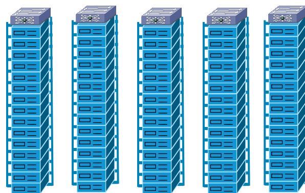
Top of the Rack (De-centralized)
