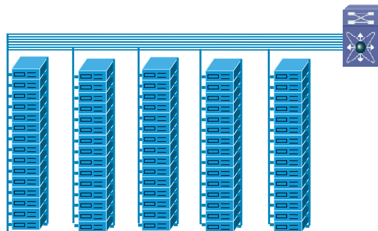
End of the Row (Centralized Server to Network cabling)
